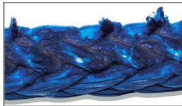
Melting or Glazing Area will be Stiff
