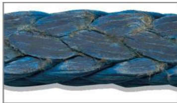
Compression Slight Sheen Is Visible
