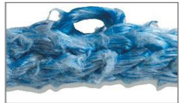
Rope Strands Reduced from abrasion
